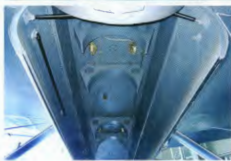
Bomb bay of Z.506 B, which was modified for loading rescue boats and other safety equipment when converted to an 'S' version
