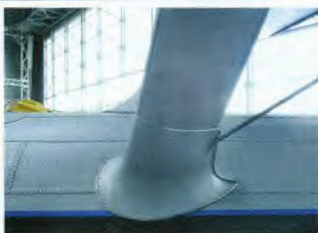
Aerodynamic fairings cover the strut connections to the floats
