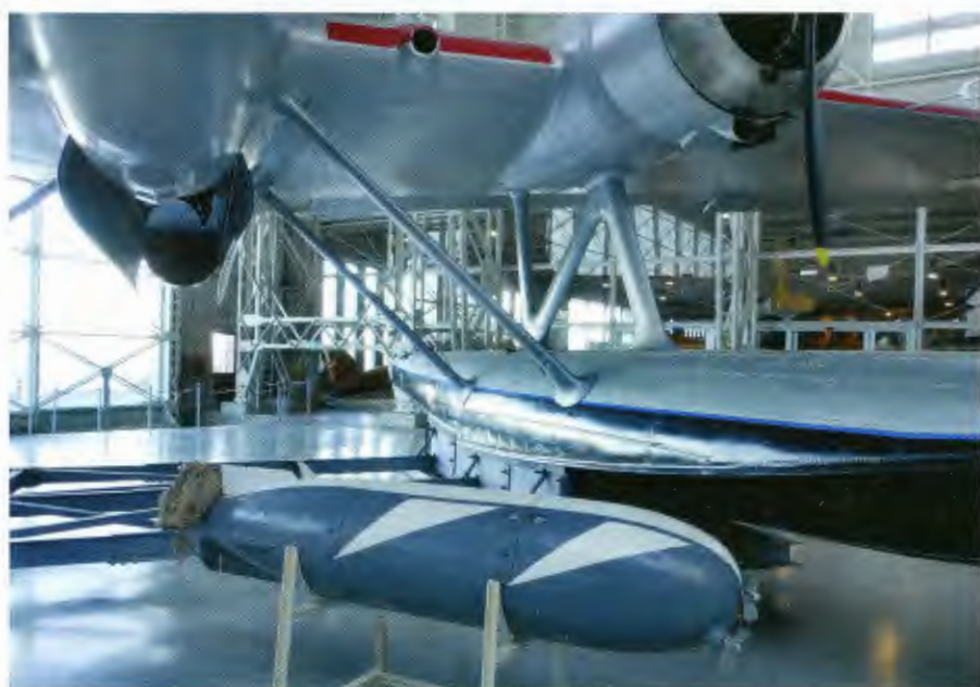
One of the two bombs normally loaded on the Z.506 B, and details of the struts connecting the floats to the fuselage
