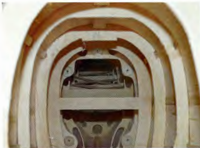
ABOVE: Fuselage frames are made from poplar plywood, covered in balsa
